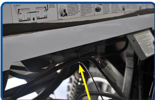
Tie the wiring harness to the main harness at the back of the battery compartment as shown.
