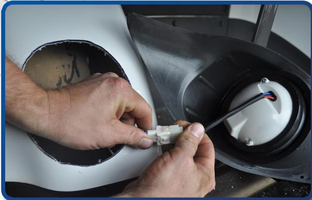
Route wiring harness behind rear fender wells. Connect tail light to wiring harness and mount to body using supplied fasteners.
