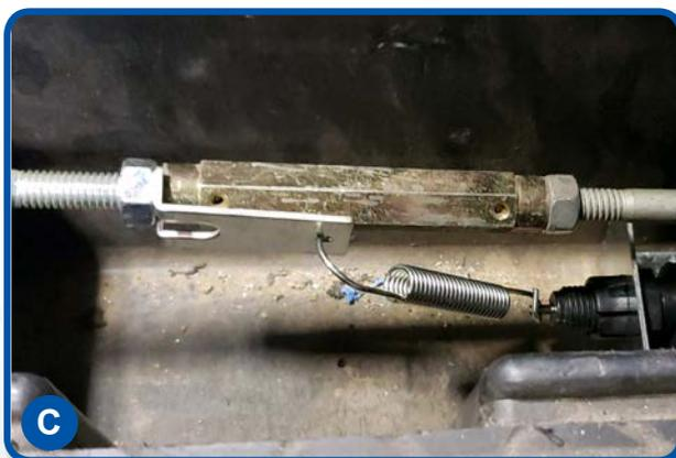
Loosen lock nut on brake rod. Place the forked bracket around the brake rod behind the lock nut and tighten the lock nut sandwiching the bracket. Place the brake switch on the floor of the car with the spring running towards the back of the car to the brake switch.
