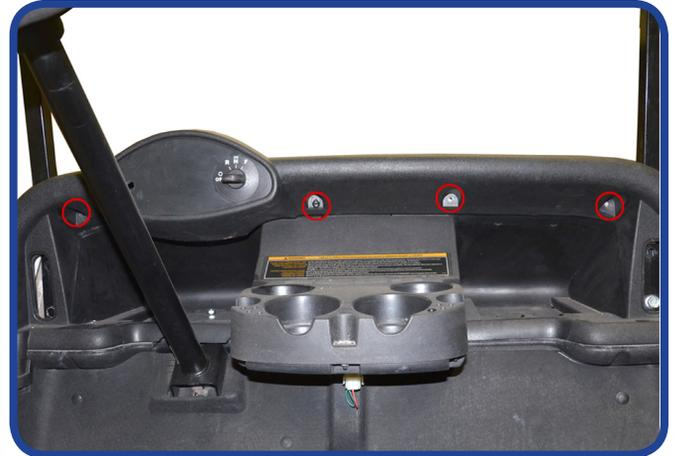
Unscrew torx-head screws and remove dashboard. Retain hardware. \*Do not remove completely.
