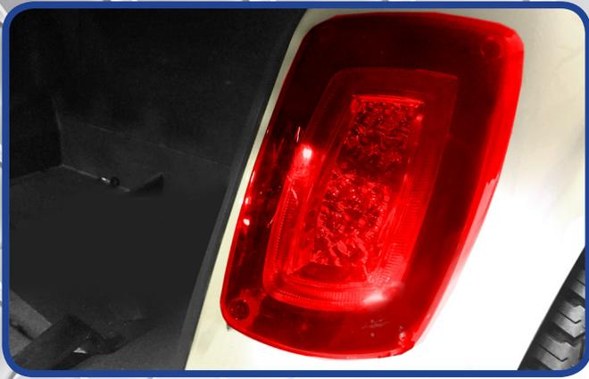
Place tail light into the rear of the vehicle. Insert four screws into Tail light using supplied hardware.
