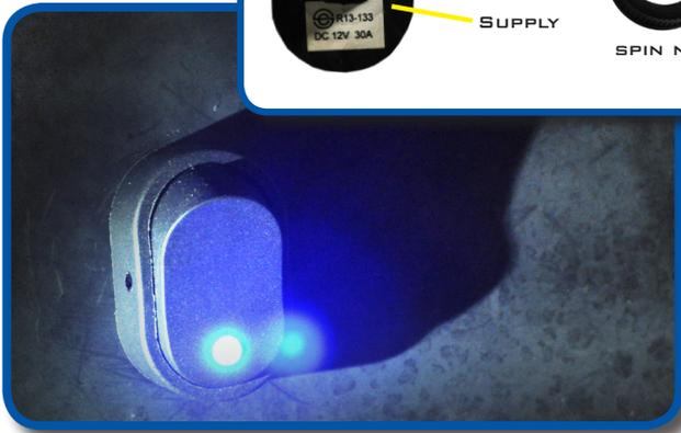
Using a 15/32" drill bit, find a desired location on your golf cart dashboard to mount your rocker switch for hazard lights. Ensure your location is free of obstacles and will not affect dash reattachment.
