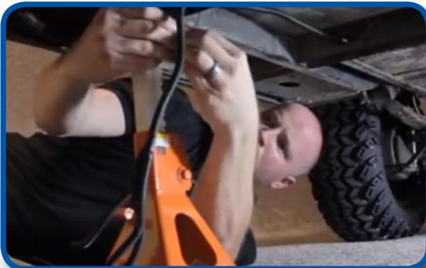
Lift the cart and place jack stands to support. Feed the headlight portion of the harness down through the front of the battery compartment. Route the wiring harness through the holes under the frame. Run long tail light wire under the seat and over the rear tire well on the passenger's side. Run short tail light wire under the seat and over the rear tire well on the driver's side. Loosely secure with wire ties until all lights have been installed.
